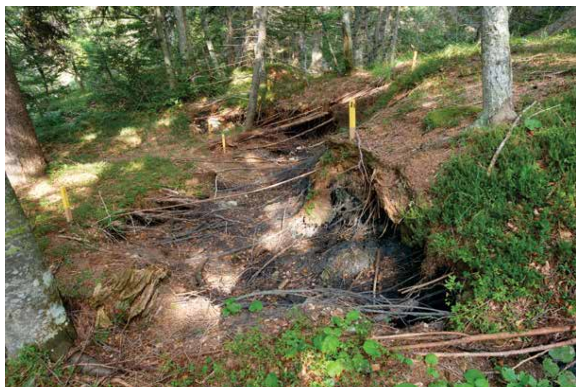
Fig. 45: Longitudinal cracks and stretching of tree roots in the Carboniferous and clastic rocks.
