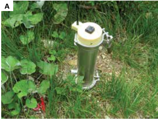
Fig. 9: A- installed GEASENSE probe; B- Locations of GEASENSE probes (Verbovšek et al., 2017a).
