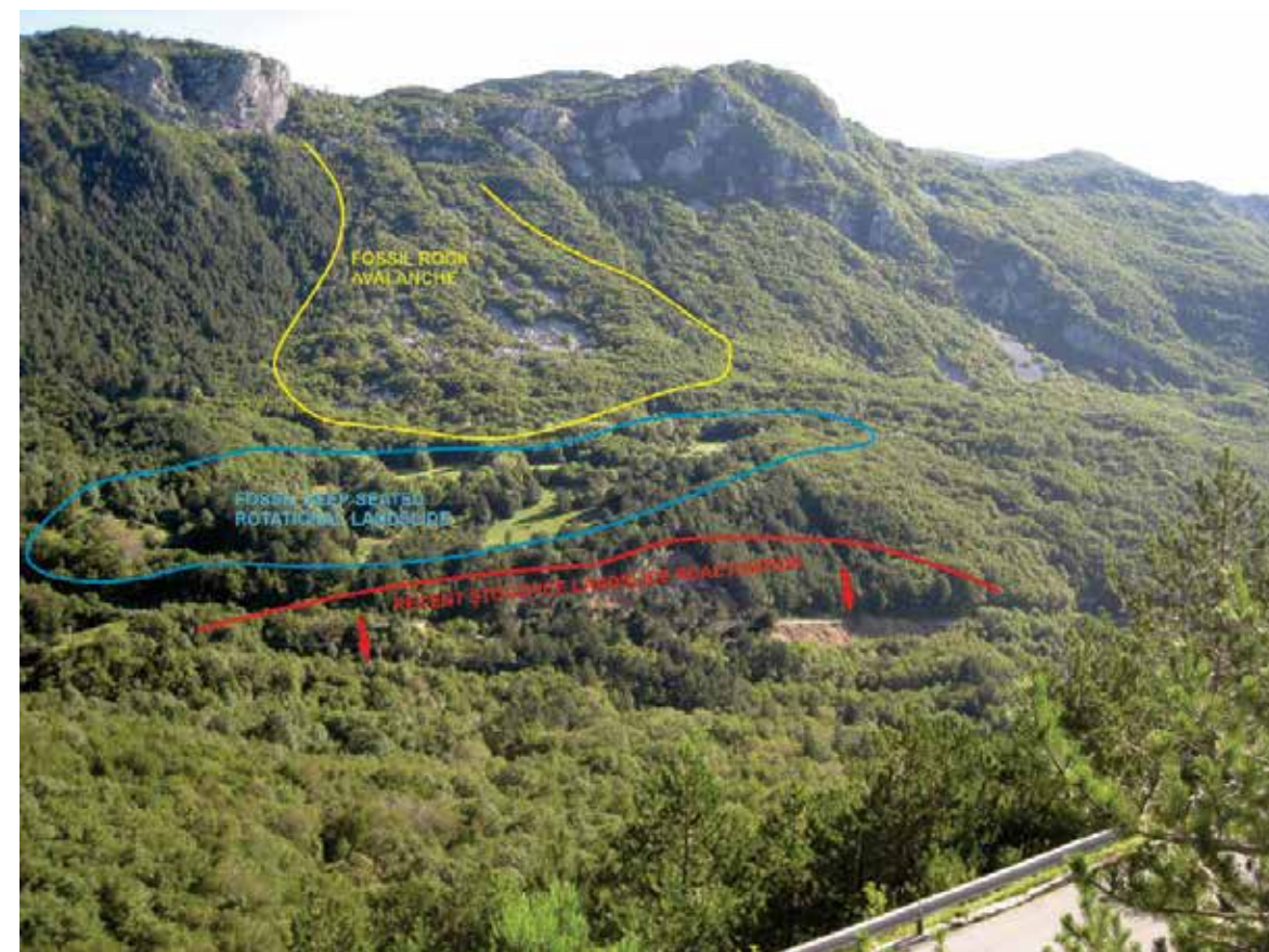
Fig. 8: Interpretation of Stogovce landslide, older fossil landslide in the upper part and more recent activation in the lower part.
